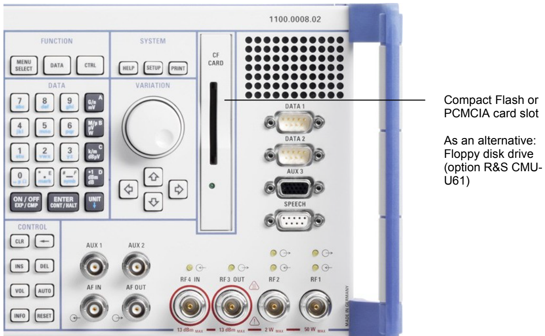
Fig. 1-7 CMU front view – Compact Flash card slot
